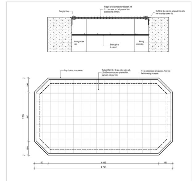
STEEL03 STEEL GRILLE TO OPENING IN CONCRETE ROOF 1:10
