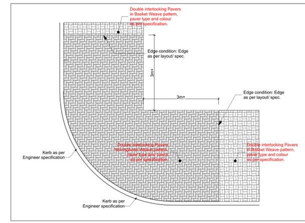
PAVE07 TYPICAL PAVEMENT PATTERN AT CORNERS DETAIL 1:50
