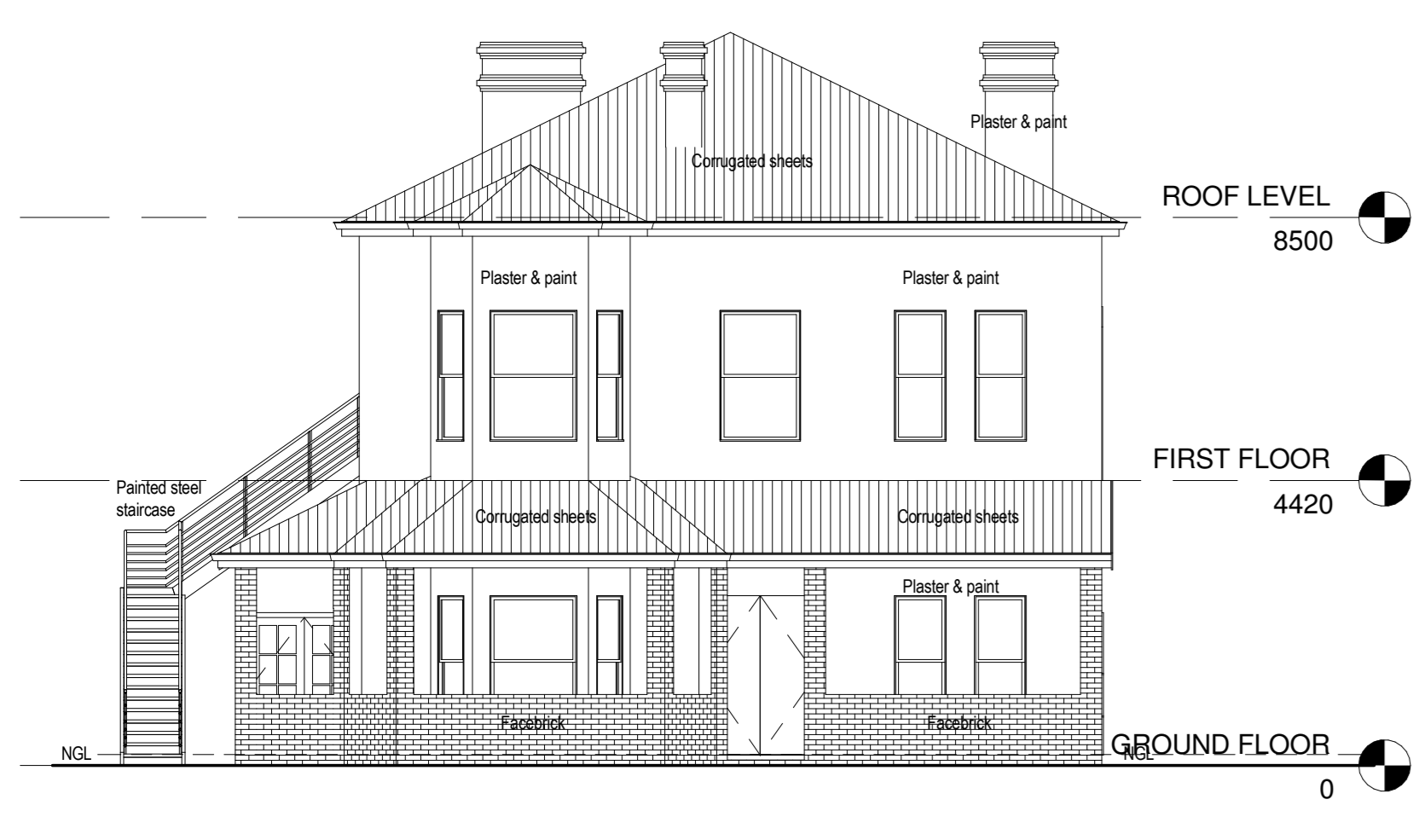
EAST ELEVATION SCALE 1:100 NOTE: PROVIDE PROVISION TO REFURBISH EXISTING BURGLAR BARS ON ALL WINDOWS
